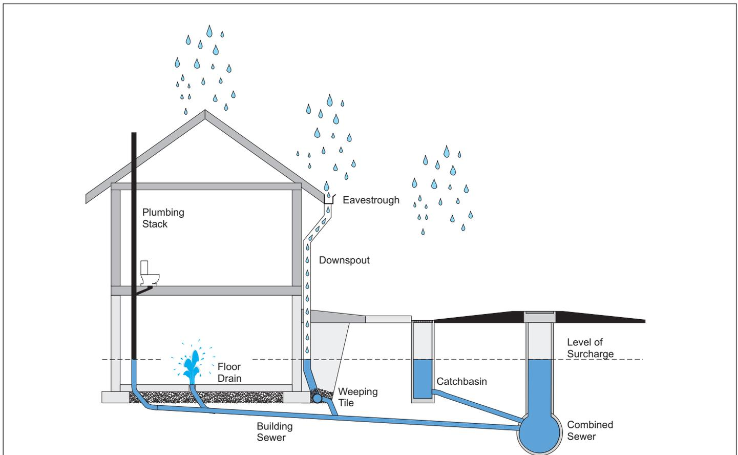
**BASEMENT FLOODING DUE TO COMBINED SEWER BACKUP**
