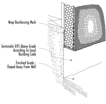
Fig. 1 WRAPPING - Alternate 1 Fiber mesh located between substrate and insulation is attached either by base coat.
