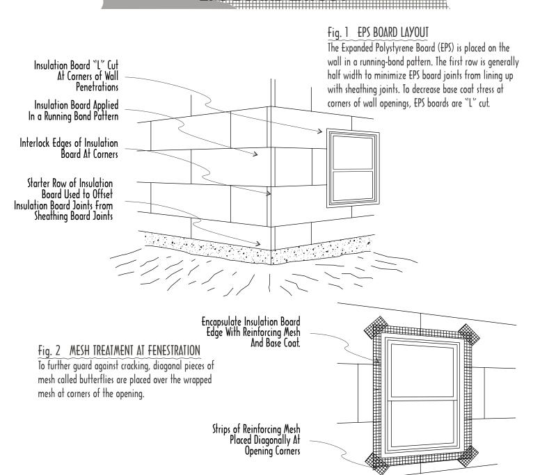
NOTE: Window flashings, not shown, are placed at the head and sill.
